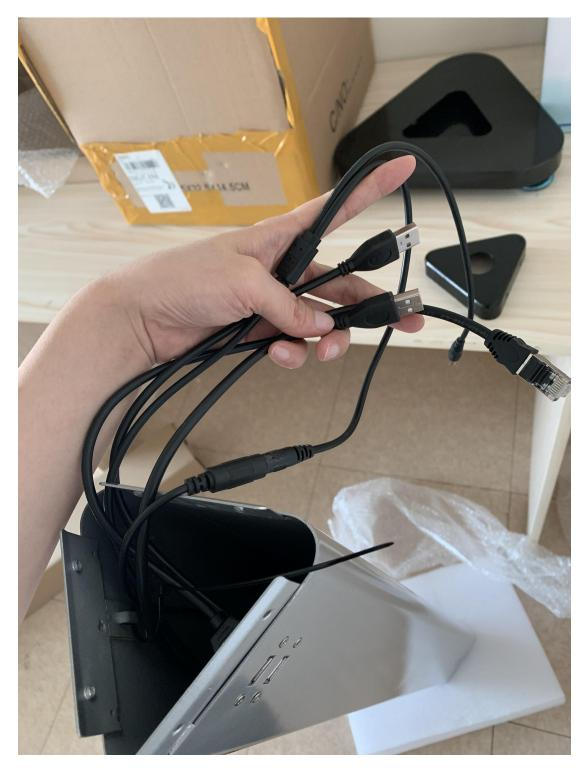
7. Connect the device's cable with the floor stand's internal cable
