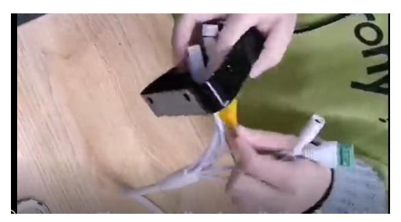
6. Put the device's cable through the black part's hole.
